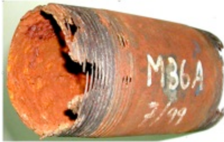
Figure 4: Corrosion failure of the material.
