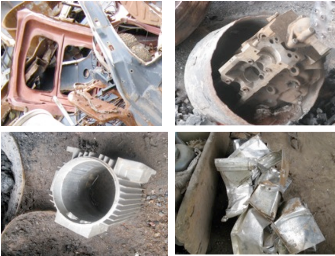
Figure 3: Aluminum containing scrap used for cooking pots. 3
